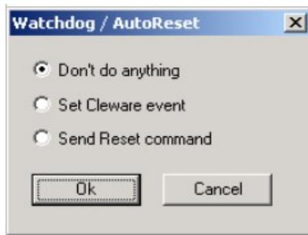
If "Set Cleware event" is selected, an error event named "ClewareControl" with the event number 16 is entered into the event log when the Ok button is pressed. If the selection was "Send Reset command", the reset command will be send immediately to the guard.
