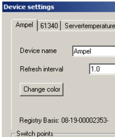
The properties of every Cleware USB device is stored in registry at "Cleware GmbH->USB" in several key value pairs. The name of all keys start with an unique device identifier, the Registry Base. This unique identifier is displayed in the device setting dialog.
