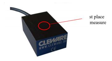
To get the best results, the object to by measured should be placed at the position shown above. The sensor is thermical connected with the aluminium housing so changes in temperature will cause an immediate reation.
