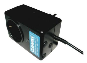
The USBwatchdogXP uses an opening relais. Without intervention the mains socket is supplied with current. If the current should be interrupted this is done by turning the relais on.. Next to the socket a LED is located to indicate the switch state. The LED is green if the PC is running and red if the a malfunction has been detected and the switch is active. When the USB-Watchdog XP waits longer than 10 seconds for service the LED turns to yellow to indicate a kind of prealarm
