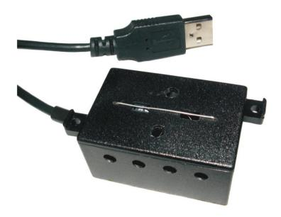
In contrast to USB-Temp, which measures though the housing, the USB-Humidity measures the air temperature and humidity directly using a hole in the middle of the housing. The dimension of the device is about  $44 \times 30 \times 23$  mm. The operating temperature should be between -20° and +80° Celsius. Using it outside this range may cause the destruction of the sensor. If temperature falls below 0° C the cable must not be moved or bent.
