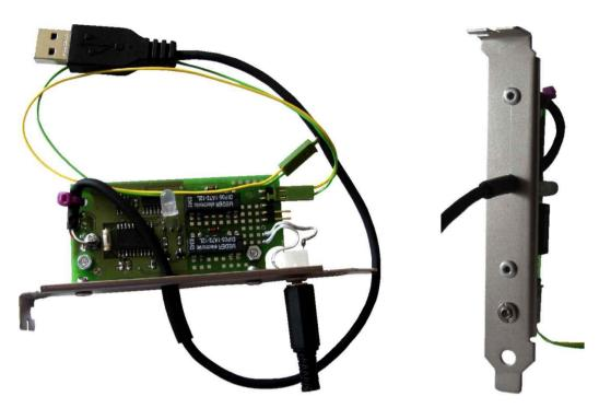
The device USB-AutoReset is also availabel as a slot version to install it inside the PC. The electronics are mounted on a slot bracket. The USB cable is about 25 cm long and placed through the slot bracket. Alternatively the USB cable could be supplied with a 4 pin plug for direct connection on the main board.
