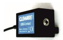
The size of the sensor is about  $44 \times 30 \times 23$  mm and it is connected to the PC using an approx. 1,8 m USB cable. The contact applies with 5 V and less than 0.1 mA. The product is guarranteed for 4 years. The valid temperature range for the USB-Contact is -0° to +80°C. Using the sensor outside this range may destroy it.
