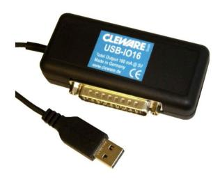
The contacts configured as output are directly connected with +5V when turned on. When this output is connected directly with ground, this will result in a short-circuit and a destroyed device! This is not covered by the guarantee! The circuit must be choosen in a way that the maximum current of this channel does not exceed 50 mA. The total power consumption of all output channels must not exceed 160 mA.
