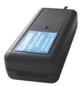
The size of the USB-AutoReset is about  $40 \times 90 \times 23$  mm. The contacts are able to switch 30 V and 0.5 A maximum. The USB-AutoReset should be operated in inner rooms only and should be protected against humidity. The permissible operating temperature range is  $10^{\circ}$  -  $60^{\circ}$  Celsius. The connection to the PC is done by the standard 2 m USB cable. On request, the device could be deliverd with a 50 cm cable and a plug for direct connection to the main board.
